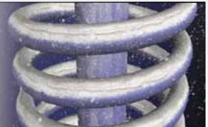
“In-tank” flue tubes and heat exchangers suffer from lime scale buildup beginning from the first hours of operation.
